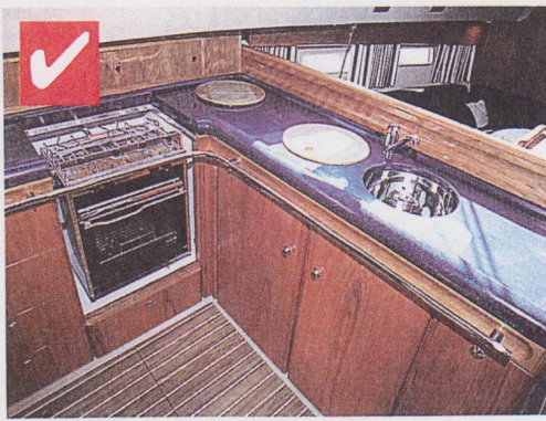
There's plenty of stowage in the galley, though the Nordstone counter needs deeper fiddles
