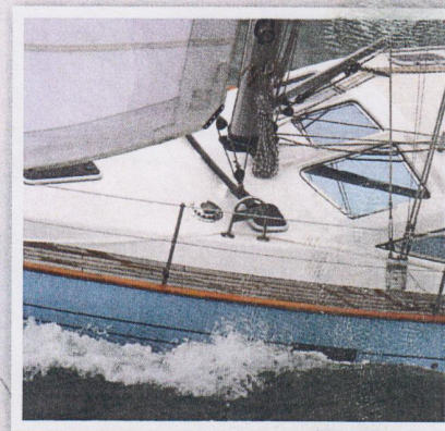
The sheet runs almost vertically from the traveller to a block half way up the mast
