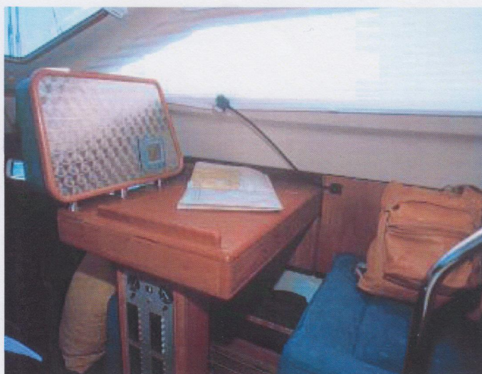
The nav desk features a clever instrument console for repeaters and a stainless steel bar to keep the navigator in place when sailing in a seaway.
