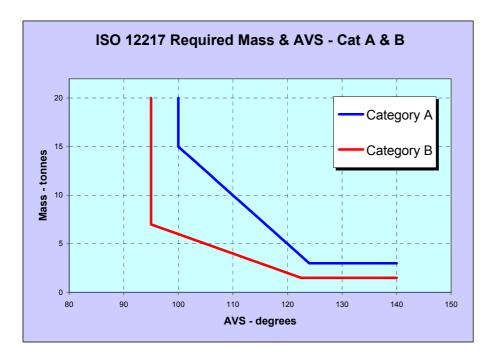
Diagrammatically this means an RCD Category A boat needs to be to the right of and above the blue line in figure 2 and an RCD Category B boat to the right and above the red line.
